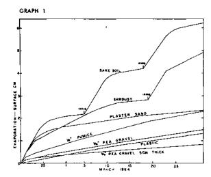
Graph 1.—Effects of various mulches on cumulative evaporation relative to bare soil, Except for the plastic sheet and the peo gravel labeled 5 cm thick, the various mulches were all 2.5 cm thick.
