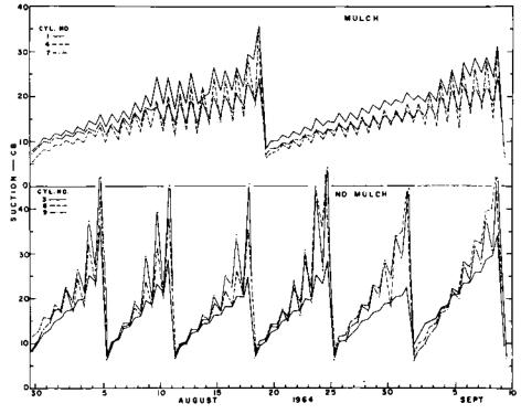
Graph 3.—Tensiometer records of suction at a 10 cm soil depth for three replicated citrus seedlings growing with and without porous block mulch. Two irrigations with mulch were equivalent to six irrigations without mulch.
