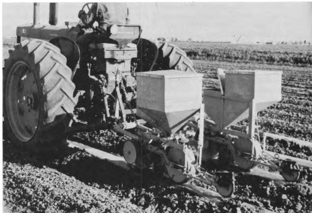
Planter used with plastic mulches. This planter punches a hole in the plastic and plants the seeds with treated vermiculite.
