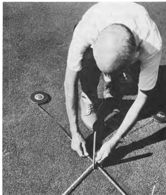
The experimental putting green was checked daily for the occurrence of "dry spots." When found, they were marked, then located by measuring from permanent reference points and plotted onto a 1:100 scale map.
