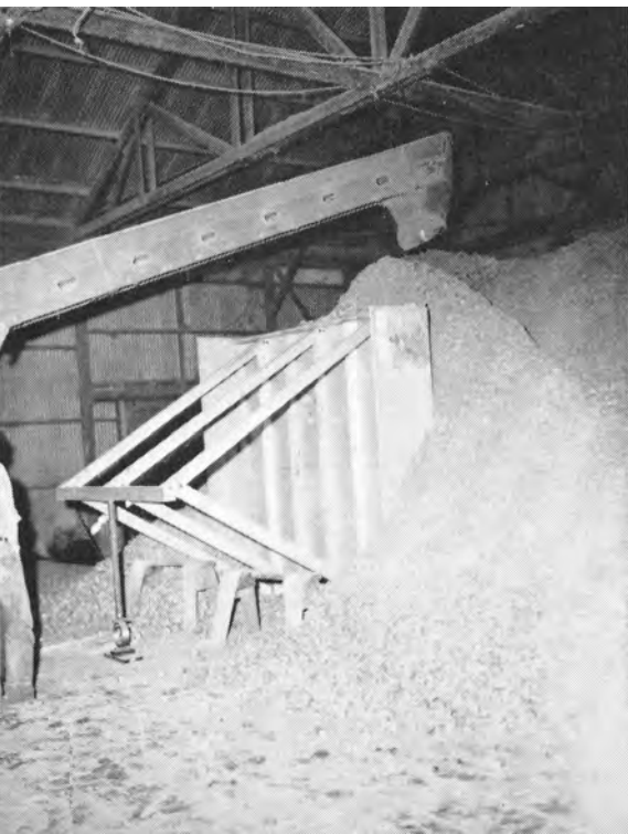
Pressure wall (8 × 8 ft) used in first test.
