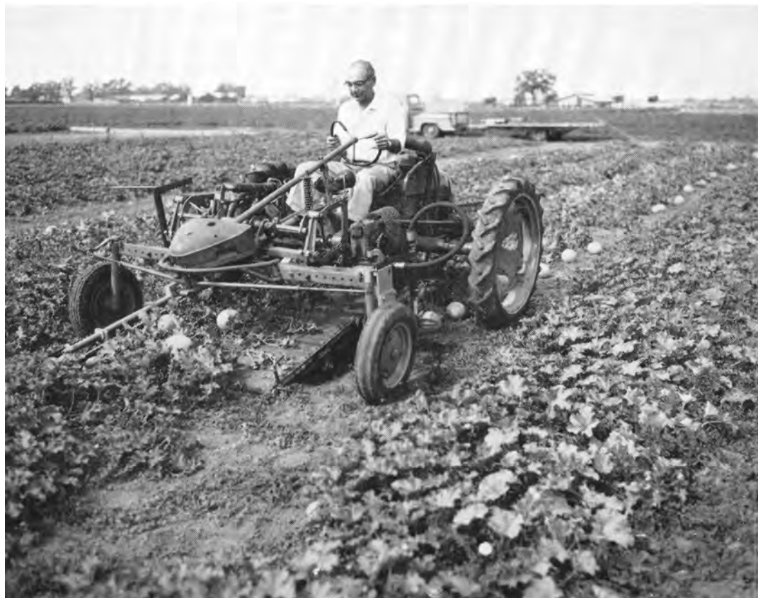
Basic elements of an experimental, selective, mechanical harvester for cantaloupes, shown in the Department of Vegetable Crops field plots at Davis. The melons deposited at the edge of the bed here would be elevated on a multi-row prototype harvester and deposited in containers.
