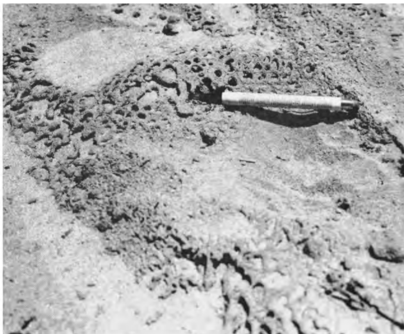
Plot above, sprayed with 1 to 3 dilution of Soil-Saver, shows untreated openings allowed the wind to remove sand from underneath the treated network, creating a bridged effect.
