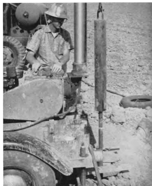
Installation of deep neutron probe tubes for the in-place measurement of soil moisture.
