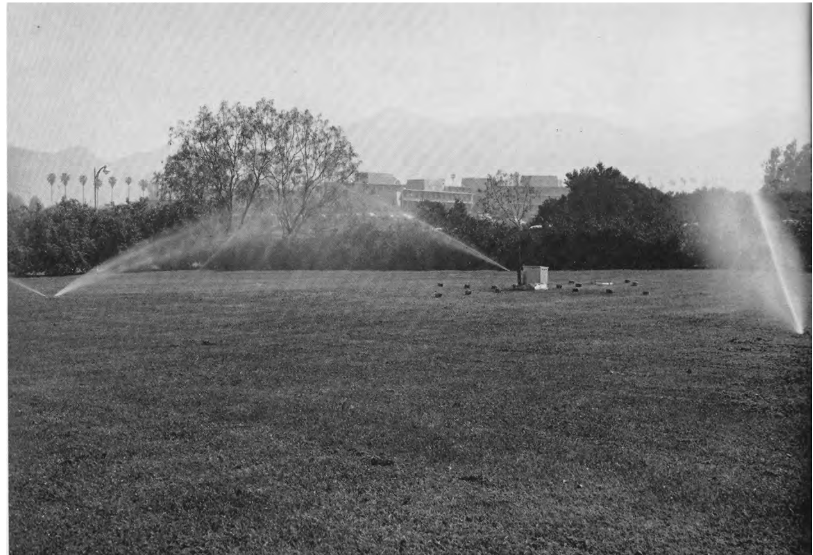
Automatic turf irrigation showing instrument area and cans set out to measure water distribution.
