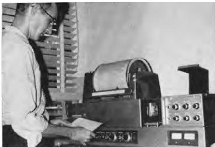
Infra-red spectrophotometer "fingerprints" an insecticide by making a graphic recording of a spectrum of a compound on punch cards for quick identification of future samples.
