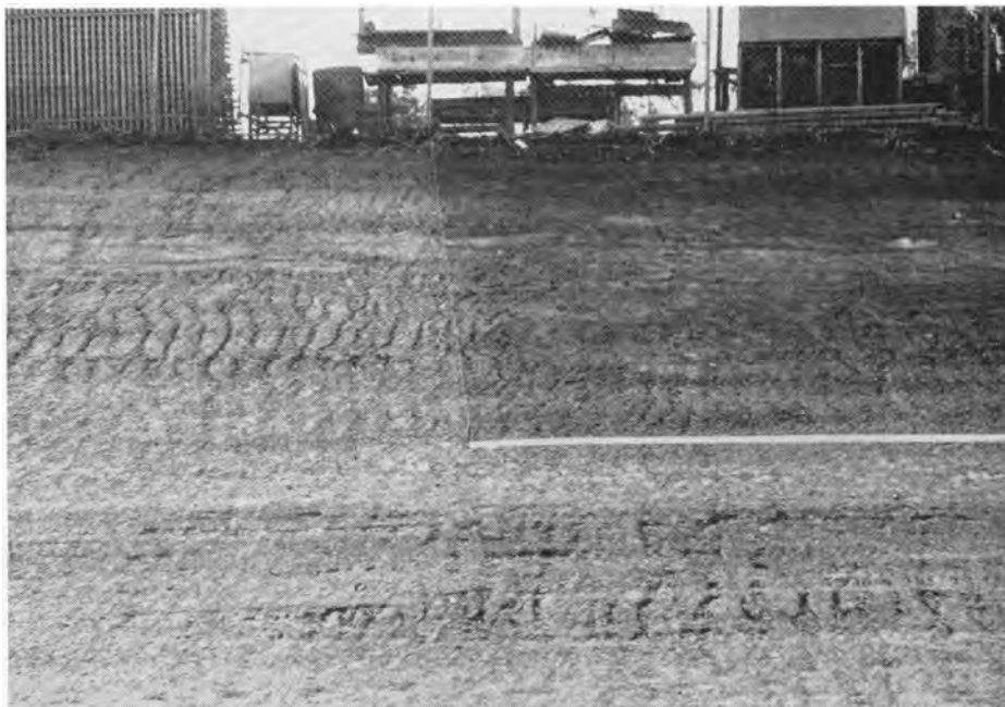
Anti-erosion test plot on 25 per cent slope following a steady two-hour rainfall of 2.3 inches.
