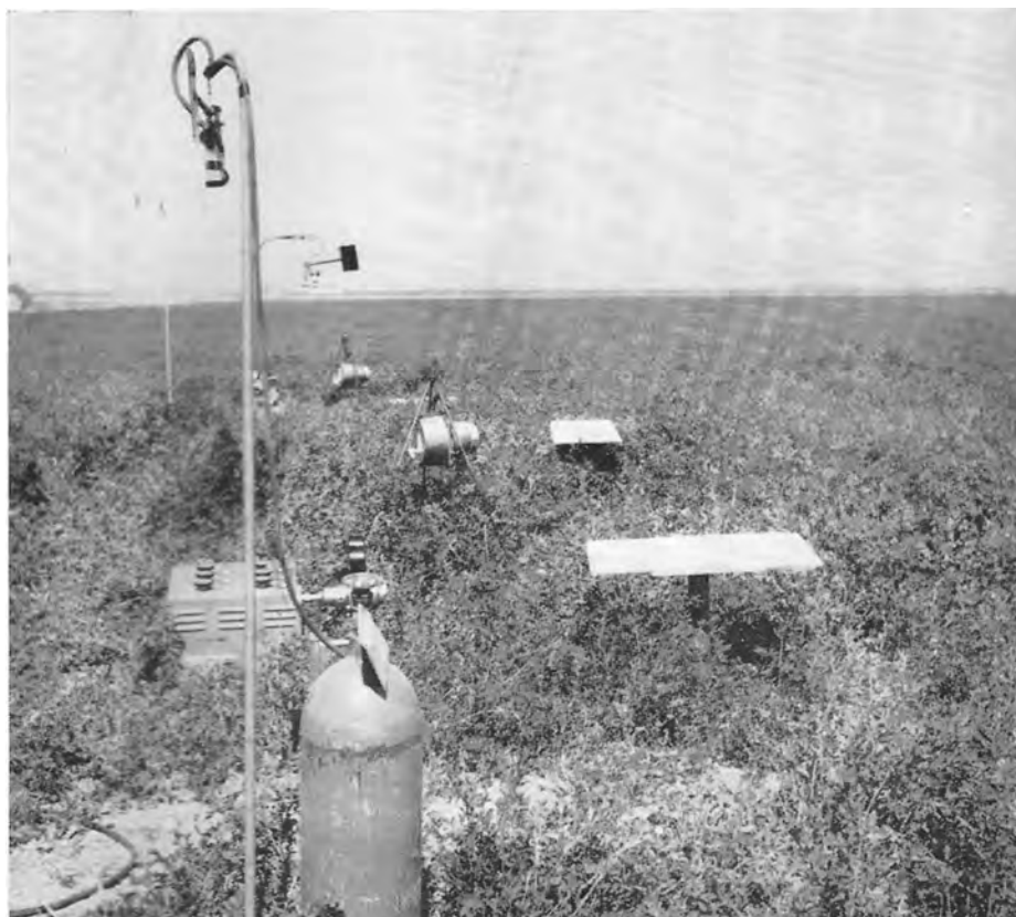
Drift sampling layout showing Cascade impactors, Staplex samplers and ground fall-out sheets.
