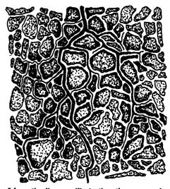
Schematic diagram illustrating the manner in which soil additives spread through small and large pores.
