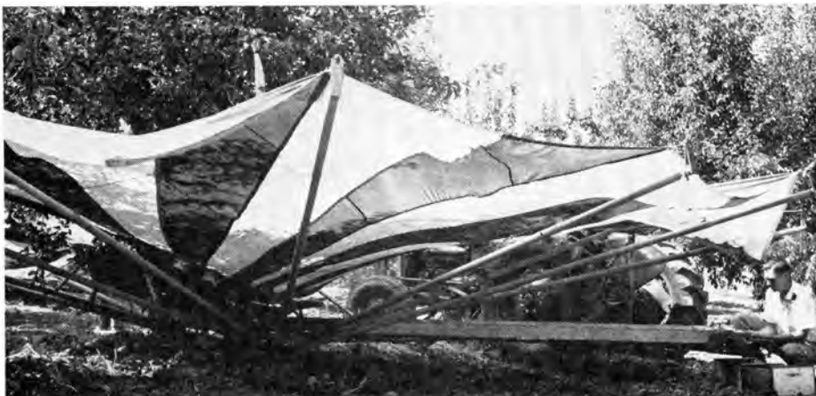
Tractor mounted catching frame in development stages used in trials with canning fruit.
