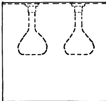
**Schematic drawing of infrared unit, showing arrangement and spacing of lamps. Wiring—not shown—is arranged in parallel.**
