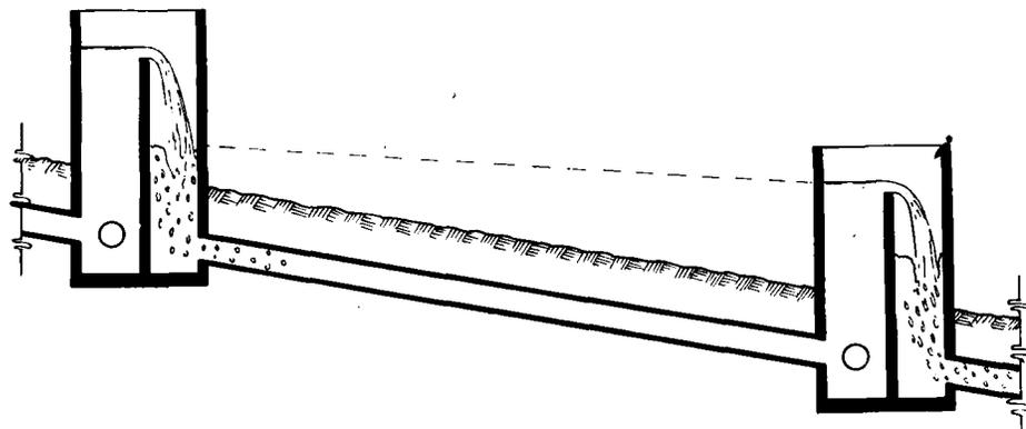
A scale model of an open system—fitted with plastic parts—permits laboratory observation of the entrainment of air, the initiation of surge, and a venting design which corrected the surge initiation encountered.
