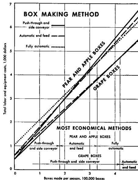
A fourth type of equipment is the fully automatic machine, which feeds the shock and nails the box. A sufficient number of machines of this type in actual use was not available for investigation. However, data based on the manufacturer's specifications were used for an approximate comparison with the more common types of equipment.
