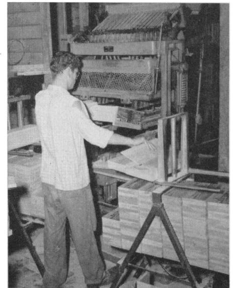
Making grape boxes on a standard box making machine with the operator pushing through finished boxes onto a roller conveyor.
