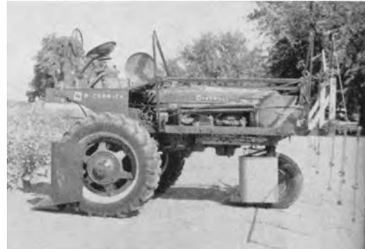
High-clearance cotton picker tractor equipped with wheel shields and sprayer.
