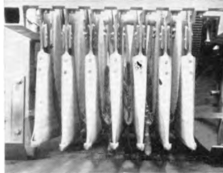
Close-up front view with harvester removed from tractor. Each pick-up unit covers 2½" of row width. Note spears of various lengths and diameters being held by grippers.
