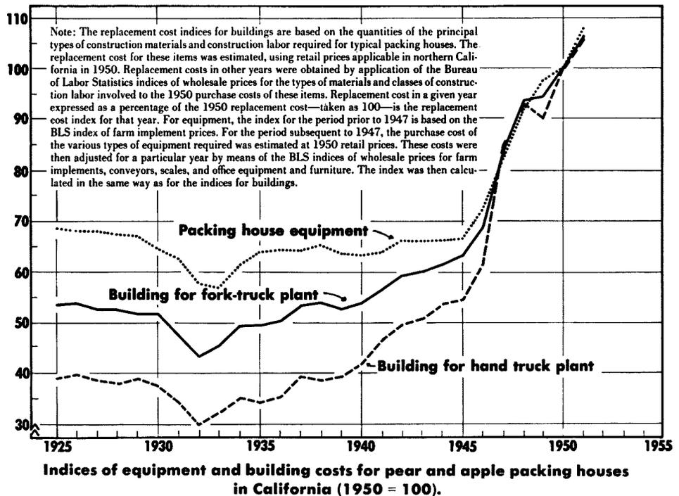
cost index for this type of construction is given by the diagram as 54. This indicates that the replacement cost in 1940 would have been 54% of the 1950 cost, or approximately \$40,500. Similarly, the construction cost index for the fork-truck plant in 1951 is 107, and the replacement cost in 1951 is 107% of the 1950 cost, or about \$80,000.
