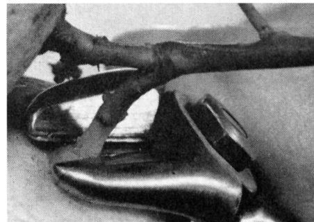
Close up view of cutting action of new lemon clipper.
