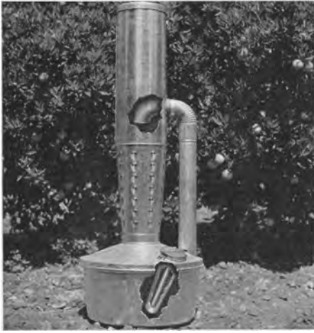
Photograph of the Return-Stack orchard heater with cut-away drawings to show interior details.
