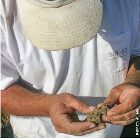
Co-author Toby O’Geen investigates evidence of soil compaction, which can occur on trails and loafing areas where livestock congregate. Soils are especially prone to compaction by excess traffic when wet, and compacted soils are prone to erosion.
