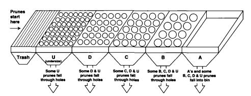
Fig. 1. Dried Fruit Association prune grading system.
