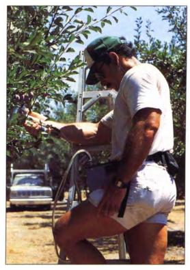
Dave Goldhamer uses a steady-state porometer to measure leaf stomatal conductance, an indicator of CO, assimilation.
