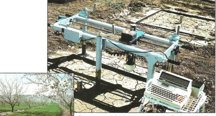
Above, a computer-controlled micropenetrometer measures the soil's surface strength. At left, a cover crop grows between the rows of an almond orchard. Herbicides have been used for strip control of weeds within tree rows.
