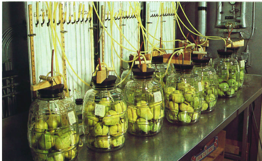
Classic experimental apparatus still being used effectively to measure fruit respiration and ethylene production and the response to modified atmospheres, temperature changes, or other "external" variables.
