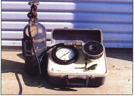
Portable pressure chamber for measuring leaf water potential is small enough to be handcarried to measurement site.
