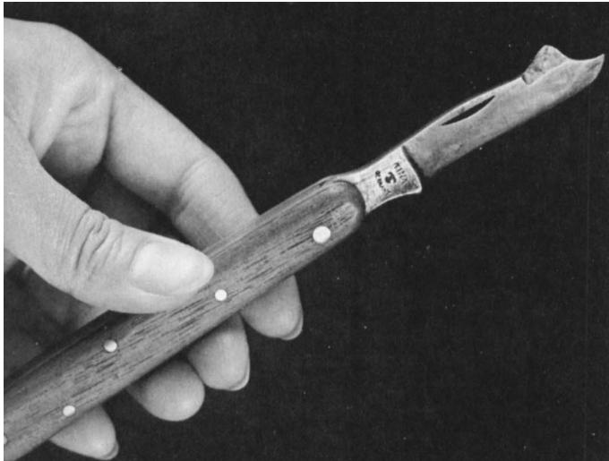
Fig. 1. Knife used for T-budding. Note high point (quill) just above curved point.
