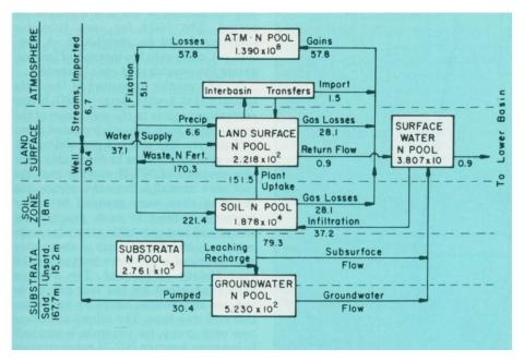
Nitrogen pools and fluxes within a 1,771,750-hectare unit in the lower San Joaquin Valley, based on the 1971 level of development. Masses of nitrogen in the pools and the numbers near the pathways that represent fluxes of nitrogen between various pools are in thousands of metric tons per year.
