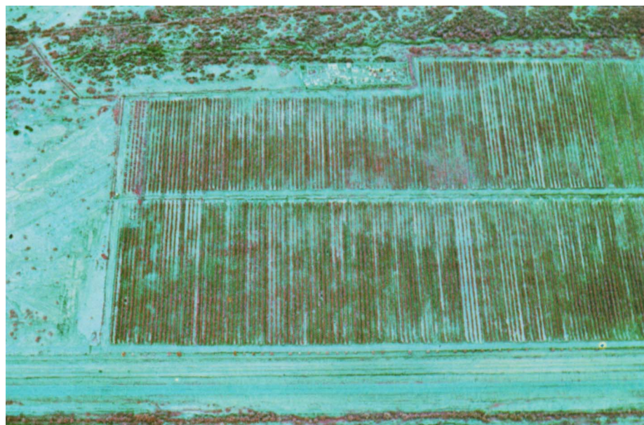
Fig. 5. Diagnosis of a vineyard problem was made by taking aerial photos a few days after flood irrigation. Small vines at the ends of the rows correlated with dry surface soils, while large vines at the centers correlated with soil that was still moist at the surface. Apparently improper leveling allowed most of the water to infiltrate the centers.
