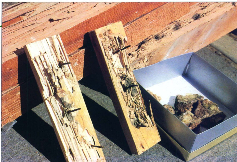
Damaged beams and Formosan termite carton (nest) in box.
