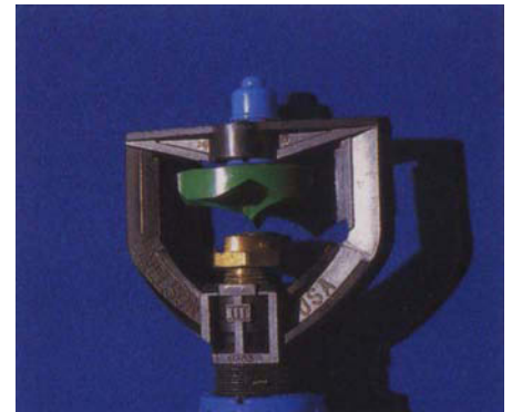
Below, the Rotator sprinkler design is similar to the spray sprinkler except that the deflector plate rotates, driven by the nozzle jet of water.
