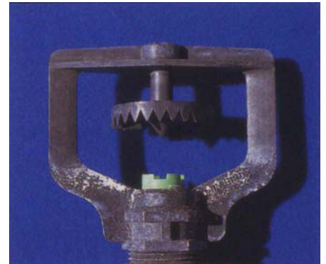
Above, the nozzle of a spray sprinkler directs water over the serrated deflector plate into multiple horizontal jets of water.
