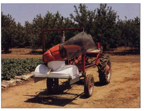
This single-bed vacuum machine, made by a grower-cooperator, uses an apple sprayer fan. It was modified in 1990 to vacuum two beds.
