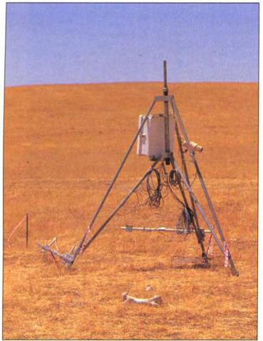
A small instrument tripod in the unirrigated grassland pasture allowed continuous measurement of surface temperature and wetness.
