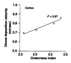
Fig. 3. Ozone deposition velocity determined by aircraft was closely related to the greenness of the plant cover determined using remote sensing from the aircraft.
