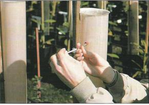
Gas sampling inside of the treeshelter with a 1-ml syringe through the septum.
