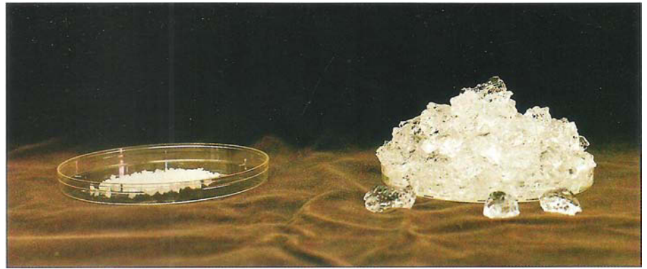
Dry polymer crystals on the left contrasted with same crystals after 130 ml of water have been added.
