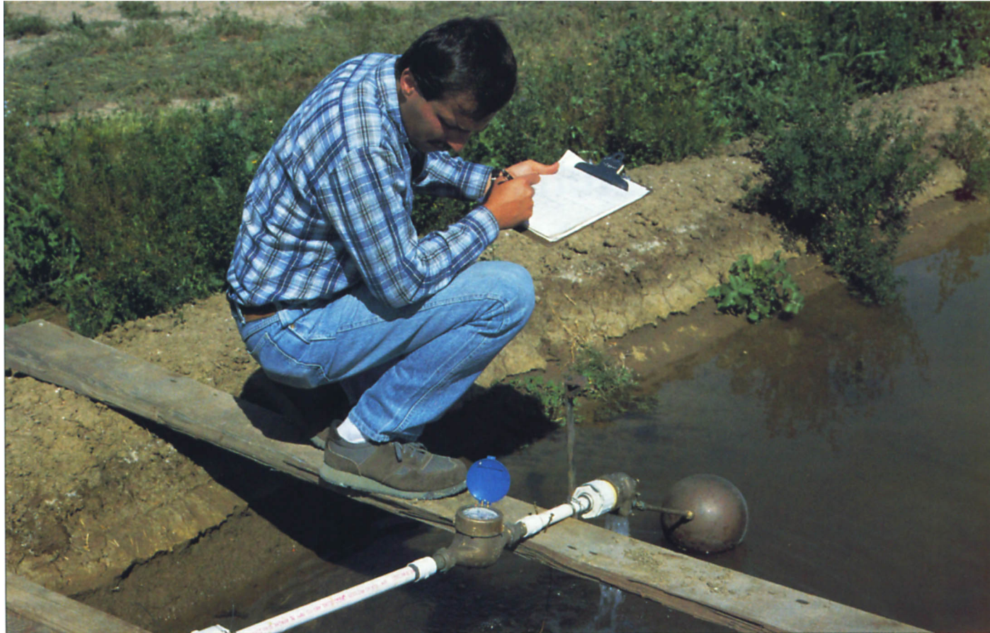
At one of the 56 test sites in the Westlands Water District, UC Davis graduate student Amir Mansoubi conducts ditch seepage evaluations.
