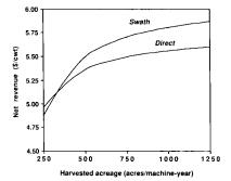
Fig. 3. On small acreages with low equipment utilization, equipment costs for swathing may exceed the benefits, up to a break-even point of about 300 acres.
