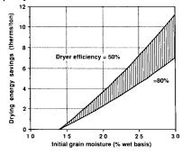
Fig. 4. Field-drying to 14% moisture could save 4 to 6 therms of energy per ton, depending on efficiency of dryer handling direct-harvested rice.
