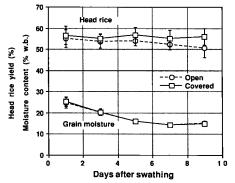
Fig. 1. Head rice yields and grain moisture, M-9 rice, 1986. Yields from covered windrows changed little but in open windrows began to drop after day 5.
