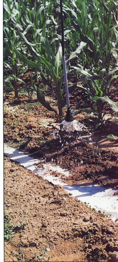
Experimental low-energy precise-application (LEPA) machine equipped with both spray nozzles (background) and drop tubes (foreground). "Bubblers" at the ends of the tubes discharge water directly into furrows (right). The system is credited in some areas with uniformities as high as 97 percent, but tests in California that considered machine movement patterns and soil intake rates showed lower uniformities.
