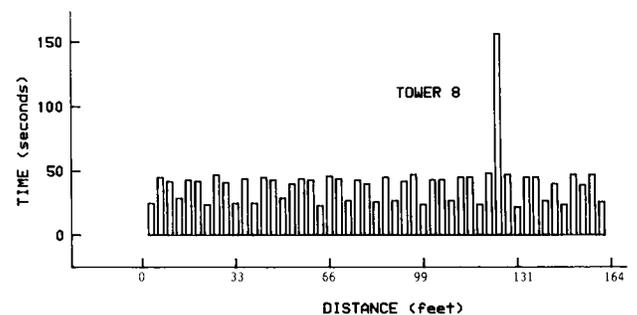
Fig. 1. Discharge opportunity times at 3-foot intervals along travel paths of two typical irrigation machine towers. Tower 8 (right) had fairly constant times, except for a large spike at about 125 feet. Tower 5 had much more variable movement times.
