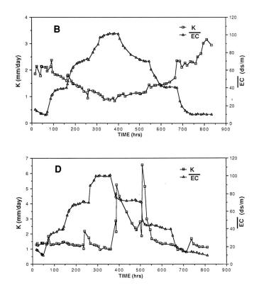
Fig. 1. When percolating drain water was nonsterile (A and B), permeability, K, decreased as mean salinity,  $\overline{EC}$ , increased. Permeability declined irreversibly as time of ponding increased (A) but rose again in relation to a
