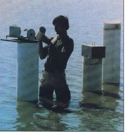
Infiltrometers (left) were installed in Kings County evaporation pond to estimate seepage. Rainfall, evaporation, drainage flows, and changes in pond water levels (here being checked by co-author Blake McCullough-Sanden) were also measured.
