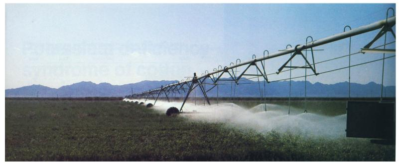
Uniformity of water application of both center-pivot sprinklers and linear-move systems, such as that above, was high near the guide towers and low near the midlateral towers. At left is the engine-powered pumping plant on a 1,300-foot linear-move machine.
