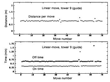
Fig. 2. Distance per move and on- and off-times of the linear-move machine showed guide tower movement to be quite constant.
