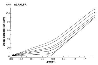
Fig. 2. Computed values of deep percolation when alfalfa is irrigated with various quantities of applied water at a given dSm. Increasing application of brackish water increases the volume of drainage water.
