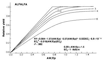
Fig. 1. Computed relationship between relative alfalfa yield and applied water (AW) scaled to pan evaporation (Ep). Each curve is for a given electrical conductivity of the irrigation water (dS/m). At a particular level of applied water, yield decreases with increasing salinity.
