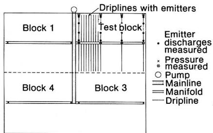
Fig. 1. Typical trickle system.
