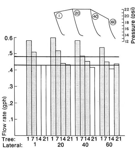
Fig. 4. Lowest quarter of discharges at ends of driplines indicates excessive pressure loss in driplines.
