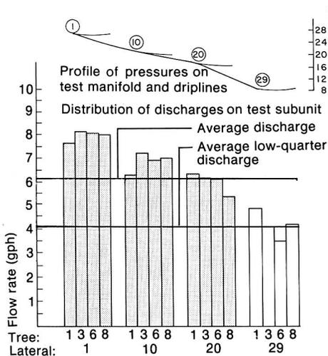
Fig. 3. Lowest quarter of discharges (non-shaded) in last dripline characterizes pressure loss within manifold.
