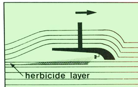
Herbicide is applied in a continuous subsurface swath as flat spray blade is pulled through the soil.
