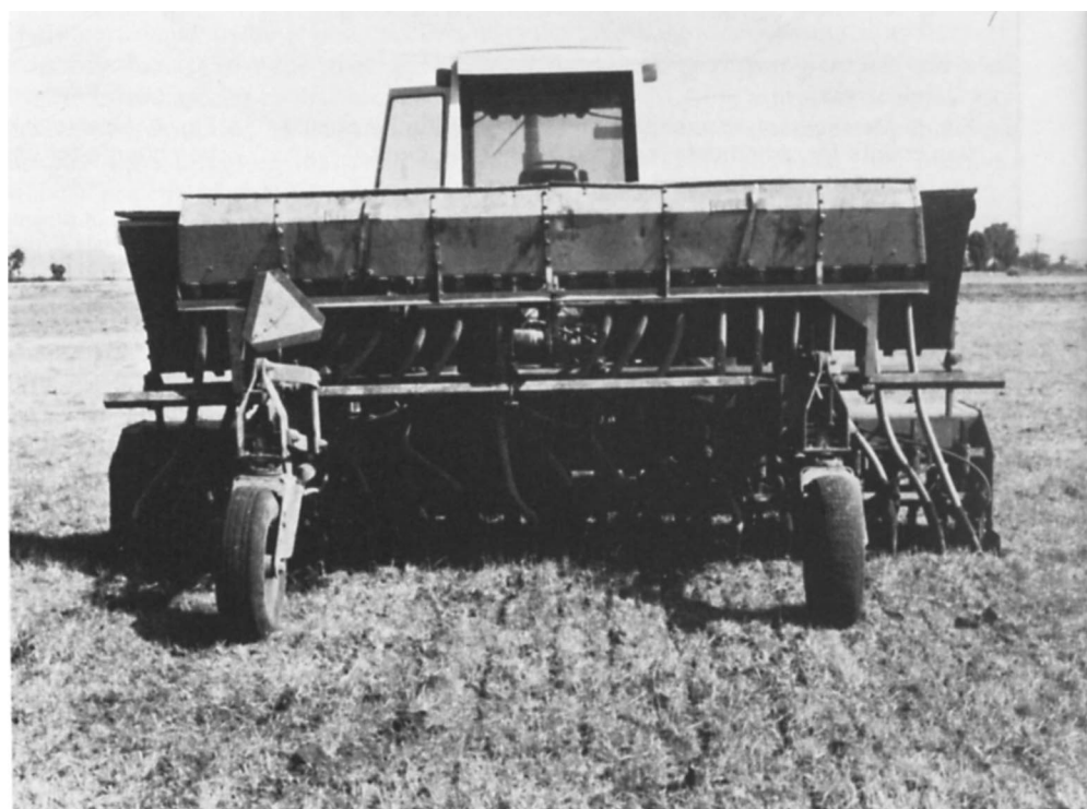
Planting annual ryegrass and applying anhydrous ammonia simultaneously to an existing irrigated pasture. No tillage is necessary.
