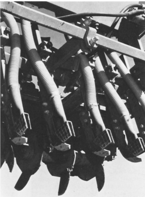
Rotating knives (bottom of photo) open the soil for backswept fertilizer shank, which applies dry nitrogen fertilizer below the soil surface.
