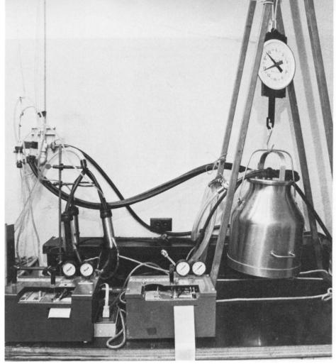
Equipment used to record milking rates and vacuum levels. One recorder charted vacuum at right front and rear teat while the other recorded pulsator action and vacuum at the claw outlet.
