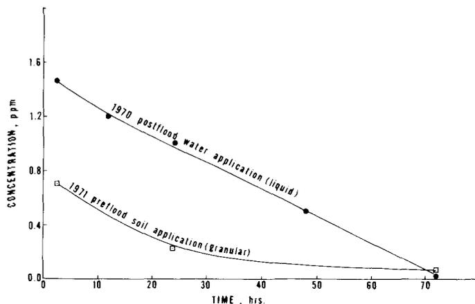
GRAPH NO. 2. 1972 DISTRIBUTION OF MOLINATE IN FLOODWATERS IN RECYCLED AND FLOW-THROUGH WATER-MANAGEMENT SYSTEMS
