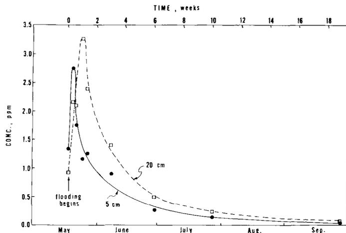
GRAPH NO. 3. 1970 AND 1971 CONCENTRATIONS OF MOLINATE IN THE SPILL-WATERS FROM A FLOW-THROUGH WATER-MANAGEMENT SYSTEM.
