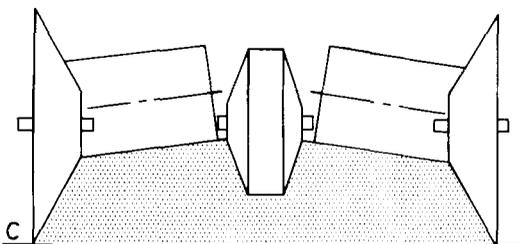
C Rolling cone press with top press cylinder for closing a reshaping experimental 60-inch bed with midbed furrow after planting.
