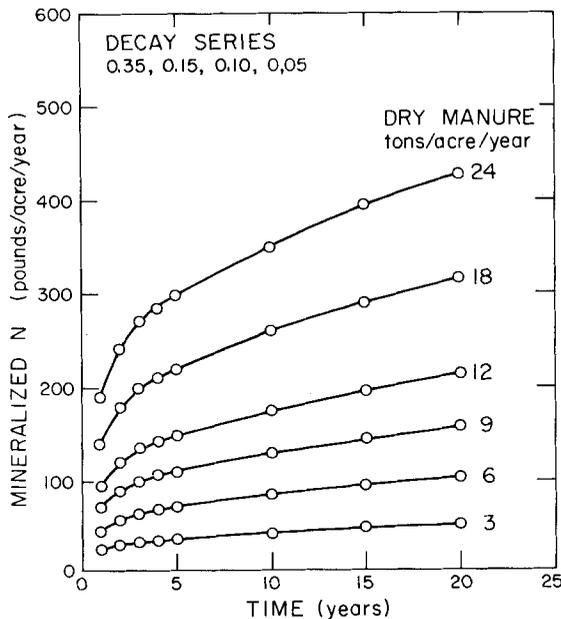
GRAPH 2. YEARLY RATES OF APPLICATION OF MANURE, CONTAINING 25% WATER AND 1.5% N ON A DRY WEIGHT BASIS, REQUIRED TO MAINTAIN VARIOUS CONSTANT YEARLY RATES OF N MINERALIZATION.
