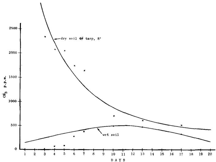
GRAPH 2. COMPARISON OF WET AND DRY SOIL IN THE PENETRATION OF METHYL BROMIDE (4 POUNDS PER 100 SQUARE FEET), AS MEASURED DOWN TO 8 FT DEPTH.
